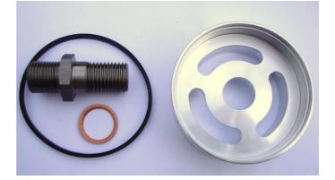
Ensure that the area around the oil pump/filter housing is clean. Remove the old oil filter container and the filter. Remove the central fixing boss and splash plate by inserting a tommy-bar through the holes in the boss and unscrewing in an anti-clockwise direction (it may be tight). Remove the old rubber seal from its groove in the oil pump/filter housing.
